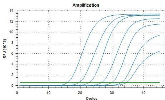
Figure 3. Dilution series of N1 target ( $10^7$ - $10^1$  copies/rxn) template run on the Bio-Rad CFX96™ Real-Time PCR Detection System (Cy5 channel).
